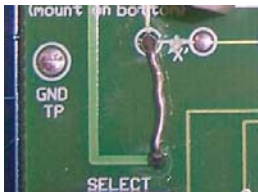
Photo 2: Adding 5V to P4 (See Assy step 8)
