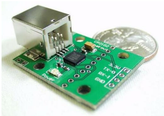
Photo 10: CP2102 USB-to-TTL interface from SparkFun
