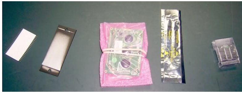
The flex cable assembly is on the left, followed by the battery cover for the case, the LCD (wrapped in anti-static padding), the IC bag and the switching regulator U9 (in a cut plastic tube mostly for mechanical protection).
