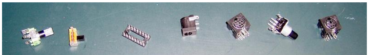
You'll need to ensure that the mini-pot (on left) and the rotary encoder (2 nd on right) get mounted flush and perpendicular to the pcb. If not, your case will not fit properly.
